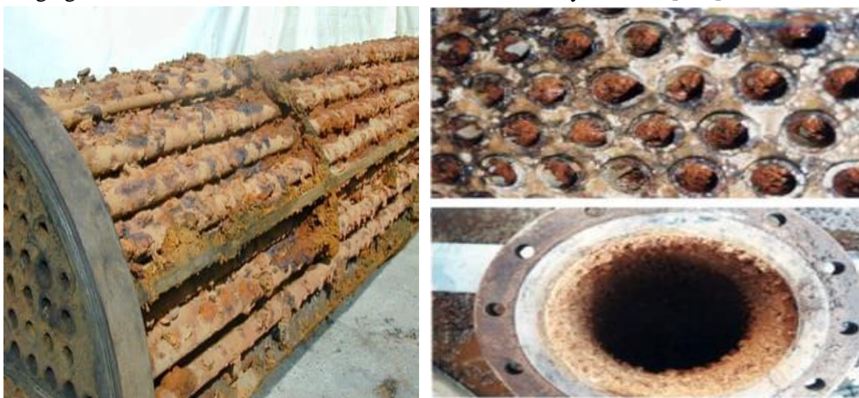
Figure 2. Failure of tubes of a shell-and-tube heat exchanger due to heat-carrying high-temperature hydrocarbons
