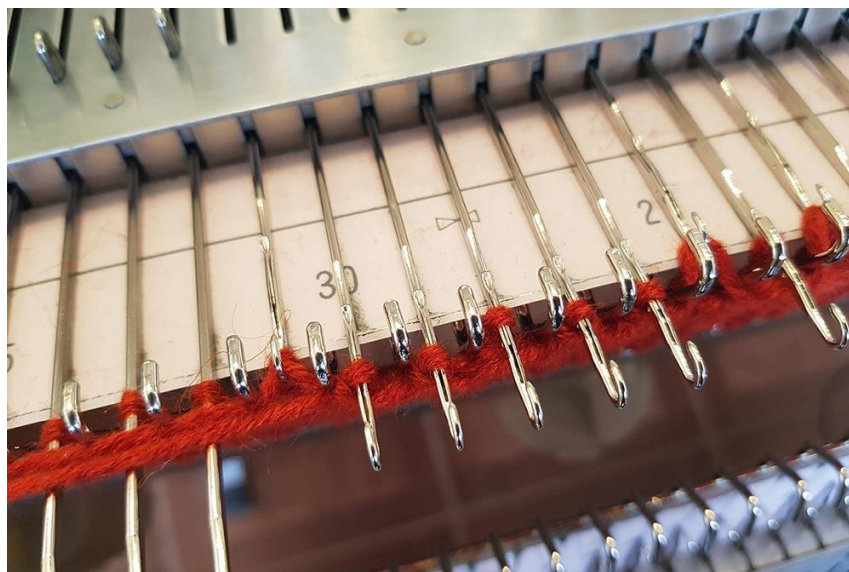
2-rasm. Yassi ignadonli to‘quv mashinasining trikotaj igna tuzilishi
